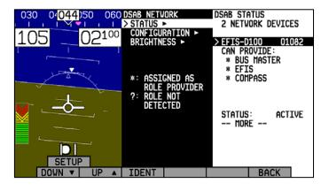
The next several lines indicate the available roles that the selected instrument can provide. A "\*" is placed next to the roles that the instrument is currently providing to the network. If any of those roles cannot be detected (e.g., the EFIS's compass has been disconnected), a "?" is displayed next to that role. Any given instrument in the list can have one of the following STATUS messages:
