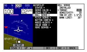
the AP should the need arise. If the servo slips continuously, the AP cannot fly the aircraft. Torque is specified in % of maximum the servo is capable of exerting. Minimum: 10%, maximum 100%, default: 100%.
