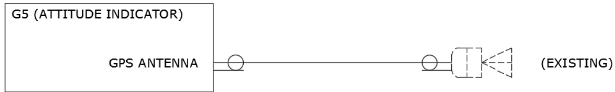
Figure 5-3 G5 (Attitude Indicator) with External GPS Antenna
