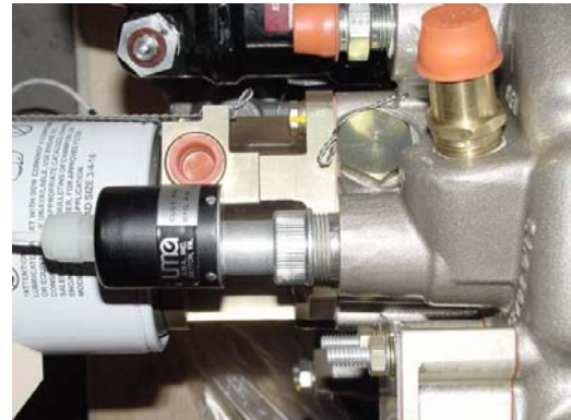
Figure 5-11. Installed Tachometer Sensor
