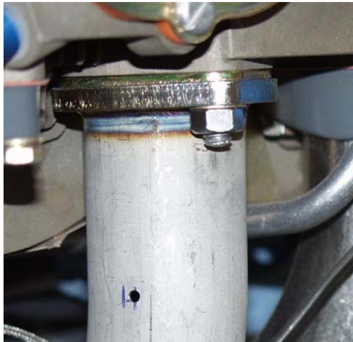
Figure 5-2. Exhaust Pipe Drilled
