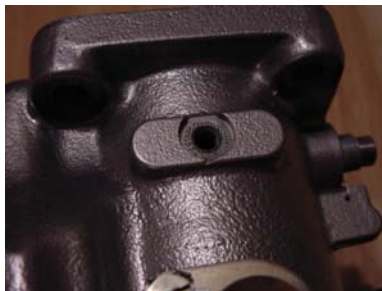
Figure 5-8. Carb Temp Sensor Mounting Location w/ Screw Removed
