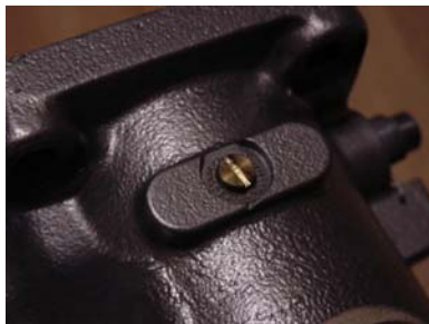
Figure 5-7. Carb Temp Sensor Mounting Location
