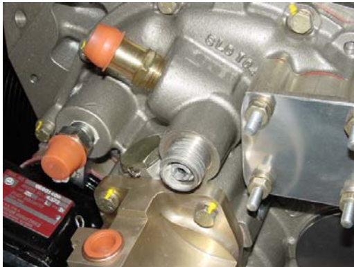
Figure 5-10. Tachometer Drive Output
