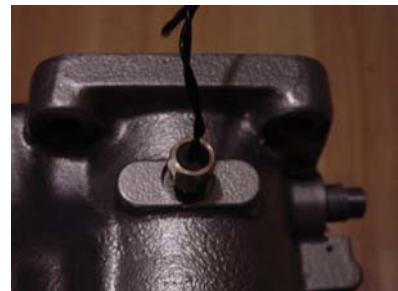
Figure 5-9. Carb Temp Sensor Installed
