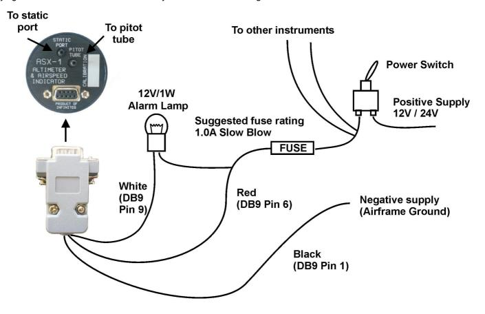
The use of an external 1A fuse is recommended. Connect the supply terminals to your aircrafts power supply. The ASI-1 can be used on both 12V and 24V without the use of any pre-regulators. Ensure that the supply voltage will not drop below 8V during operation as this may result in incorrect voltage and or current readings.
