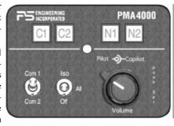
1) and "C2" (Com 2) push-buttons select the receiver, and are used to monitor a com that is not selected for transmit. You will <u>always</u> hear the audio from the transceiver that is selected by the 2-position mic selector toggle switch.
