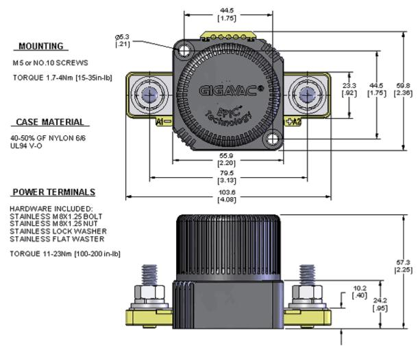
The polarity of the power terminals was previously shown reverse from what is correct and what is now indicated. The polarity is important only for switching the "Maximum Break, 2 cycles" when the voltage is over 100 Vdc.
