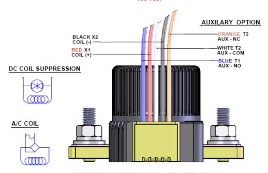
WIRE SPEC: SILICONE, 22AWG, -40C-150C, UL: VW-1
