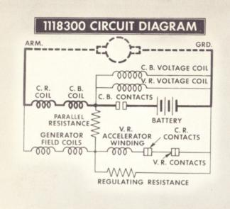
spring tension holding the armature away. The operation of these armatures controls the closing and opening of the charging circuit in the case of the relay, and the addition or removal of resistance in the field circuit in the case of a current or voltage regulator.
