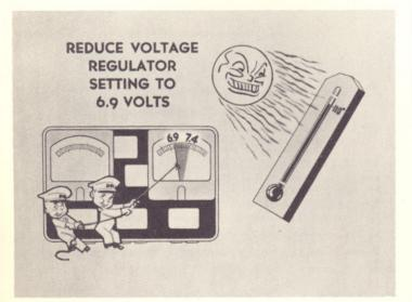
voltage regulator setting to as low as 6.9 volts in extreme cases instead of the specified 7.0 - 7.7 volts. The voltage should not be lowered for occasional trips as a normal setting would prove more satisfactory. When a reduction is made, care must be taken that the cutout relay closing voltage is approximately .5 volt lower than the voltage regulator.
