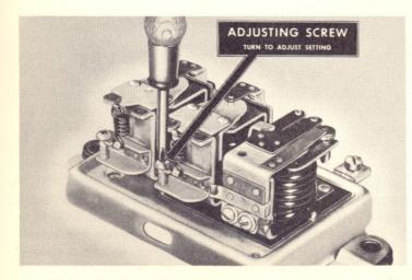
should be cleaned one at a time with a spoon or riffler file. Loosen the two contact mounting screws so that the upper contact bracket can be swung to one side; or the contact bracket can be removed if necessary.
