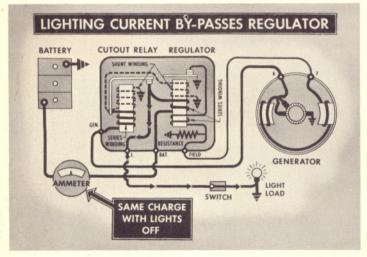
A feature of the combined current-voltage regulator is that generator output increases as the electrical load is added to the "L" terminal of the regulator. Since the load current by-passes the regulator current winding, it has no effect on the battery charging rate as long as the total load does not exceed the maximum output of the generator at operating speed.
