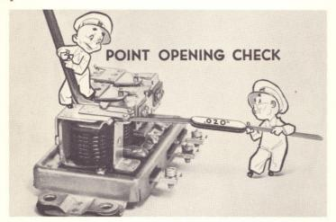
The point opening should measure .020 inch and is adjusted by bending the upper armature stop.
