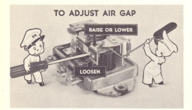
upper contact bracket as required. Make sure the points line up properly and tighten the screws well after adjustment.
