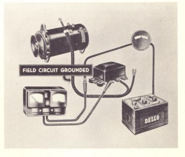
Since the cutout relay, the voltage regulator and the current regulator are mounted as one unit, it is advisable to check the entire generator regulator when any adjustment is required. A diagnosis or a system of "quick checks" readily determines whether or not the generator regulator does need adjustment, when some abnormal condition exists in the car electrical system.
