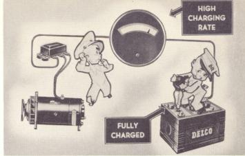
If the output then drops off, the trouble is a grounded field wire between the regulator and the generator. If
