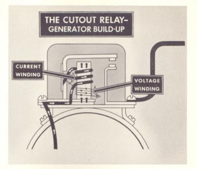
In all automotive type D.C. generator circuits, a cutout relay is used. Its points are open when the generator is not operating, thus preventing the battery from discharging through the generator. When the generator begins to operate, voltage builds up in the two relay windings, the current winding and the voltage winding, and this creates two magnetic fields which, working together, overcome the armature spring tension and close the points.
