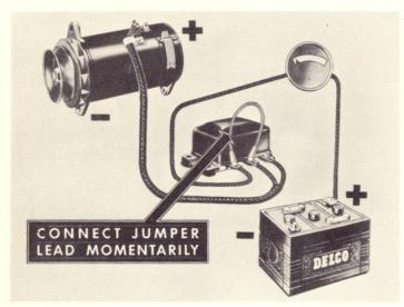
After any check or adjustment of the regulator or generator, particularly after leads have been disconnected and then reconnected, a jumper lead must be connected momentarily between the "BAT" and "GEN" terminals of the regulator, *before the engine is started*. This causes a momentary surge of current to the generator which correctly polarizes it with respect to the battery. This
