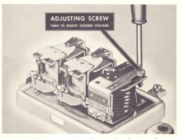
On the 1118300 series of regulators, the closing voltage is adjusted by turning the adjustment screw clockwise to increase spring tension and closing voltage and turning the screw counterclockwise to decrease spring tension and closing voltage. This is a left-hand screw.
