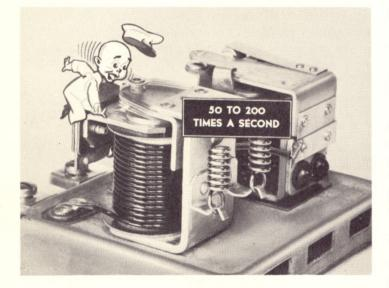
a second, causing a vibrating action of the armature which holds the voltage to a practically constant value. Any winding other than the working winding on a regulator core is used for the purpose of speeding up the rate of armature vibration, thereby reducing the amount of surge when the armature points close.
