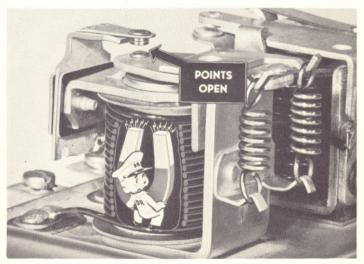
are held closed by spring tension. As the battery approaches a charged condition the system voltage increases, and the two windings build up sufficient magnetic strength to overcome the spring tension and separate the points. When the points open, the generator field current must flow through a resistance to ground, and this causes the generator output to drop off. The instant the points open, current stops flowing through the field current winding
