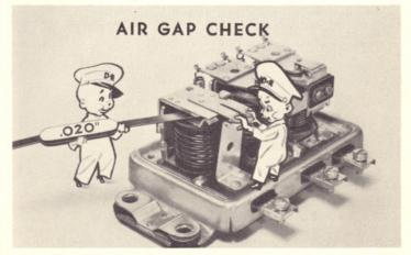
sets of points do not meet at the same instant, bend the spring fingers until they do. To adjust the air gap, loosen
