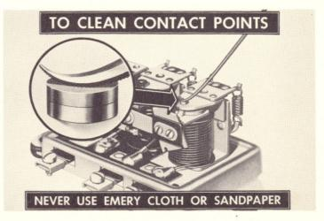
Emery cloth or sandpaper should never be used to clean contact points, since particles of emery or sand may embed in the contacts and prevent normal operation.
