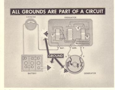
before reinstalling the regulator. The ground connections at the generator, regulator and battery are as much a part of the circuit as the wiring. Be sure a good ground exists at these units.
