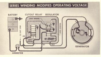
to lower the operating voltage. A high output is thus obtained only when the battery needs a charge, and the amount of charging current is controlled so that batteries are not subjected to overcharge, one of the main reasons for battery failures.
