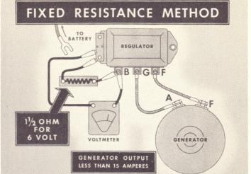
setting with the regulator at operating temperature and the generator running at a medium speed. The regulator cover must be in place. Cycle generator and repeat test.
