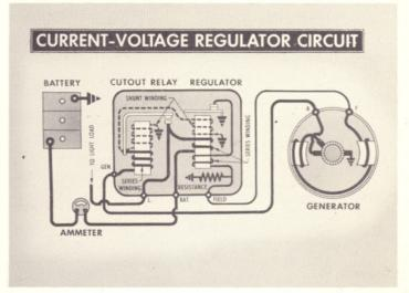
This special regulator is used in conjunction with a third brush generator which acts as a safety device to prevent excessive output when the battery is run down or improper loads are connected.
