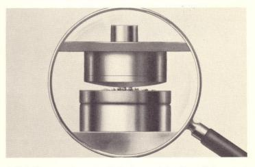
A flat file cannot successfully be used to clean flat contact points. A flat file will not touch the center of the flat point, and will not clean out the slight cavity formed in the point surface in normal operation.
