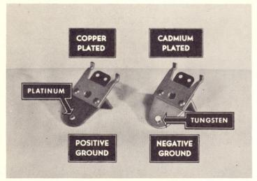
we make this point of platinum which tends to oxidize less than any other known metal. The cold side of the arc from which the metal tends to transfer is on the negative side of the circuit so we use tungsten which tends to transfer less than any other known metal. Maximum point life is obtained with this combination.
