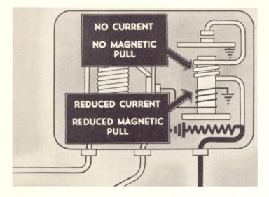
of the regulator and its magnetic field collapses. This, and the weakening of the voltage winding magnetic field as the generator output drops off, reduces the total magnetic field to a point where the spring tension once more causes the contact points to come together. The generator field circuit is thus again grounded directly, and the output increases. This cycle is repeated from 50 to 200 times
