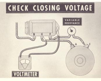
at medium speed. Slowly decreasing the resistance until the relay contact points close will also give the closing voltage setting.)
