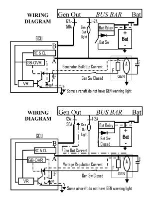
**Protection against GCU induced OV fault.** The GCU's design will cause the field current path (between the field and ground) to open and the VR switch off if the field control device becomes internally ground shorted. This means that the GCU will not induce Over-Voltage (OV) problem into the system. The GCU does not protect the system against externally induced OV faults.
