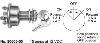
Mounting stem: 13/16" - 24 thread. Actuator: coded tumbler lock.
