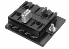
**Electrical Ratings** 25 amps max. per circuit @12 VDC 150 amps total for block @12 VDC For 24 VDC applications use only ATC or ATO fuses.
