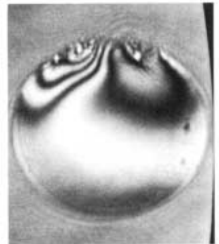
This view represents a fiber endface as viewed by an interferometer (50/125 micron corning fiber). The light/dark bands (fringes) indicate end face angle.
