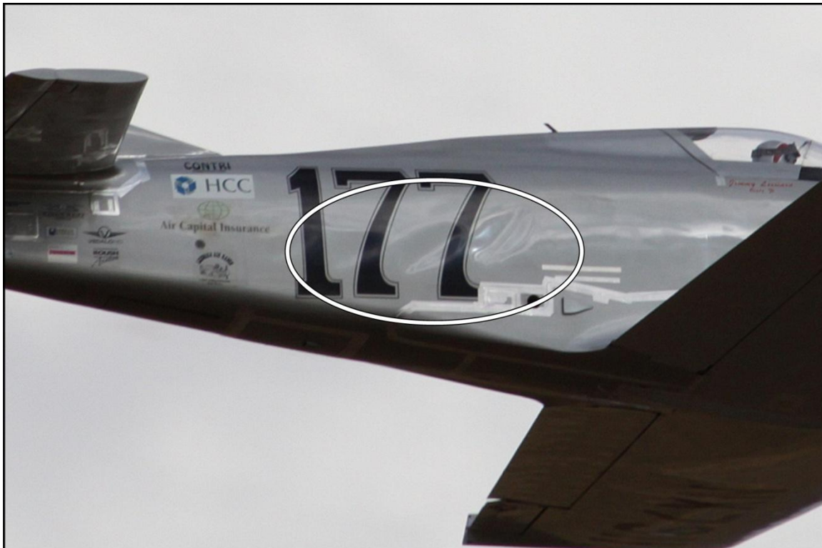
Figure 15. Diagonal wrinkles on right side during accident race.
