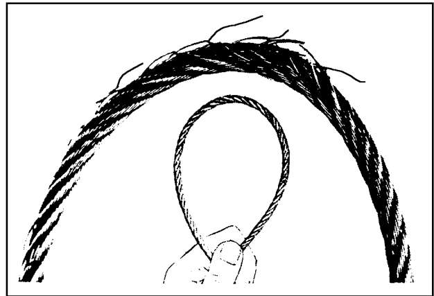
FIGURE 7-16. Cable inspection technique.
