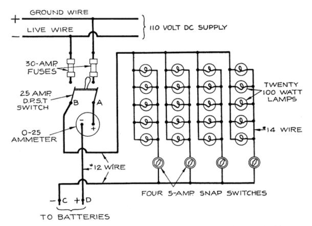
Fig. 39. Lamp Bank for Charging from a 110 Volts, D. C. Line (Positive Grounded)
