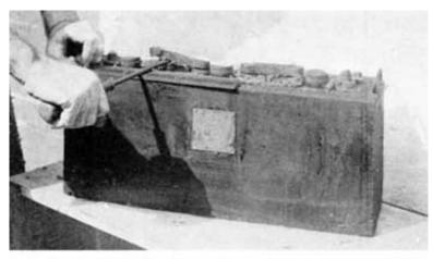
Fig. 193. Prying Off Cell Connector
