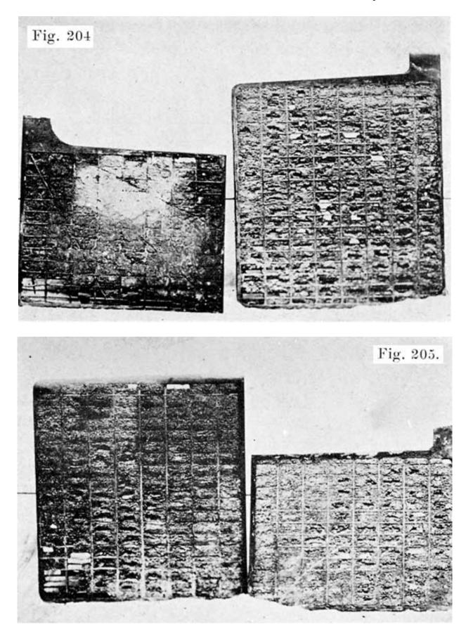
Fig. 204 and 205, Show Diseased Negatives. The Large Ones Only Eight Months Old. Active Material, Granulated and Blistered.
