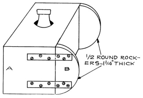
Fig. 131. A Simple Method of Drawing Acid from Carboy
