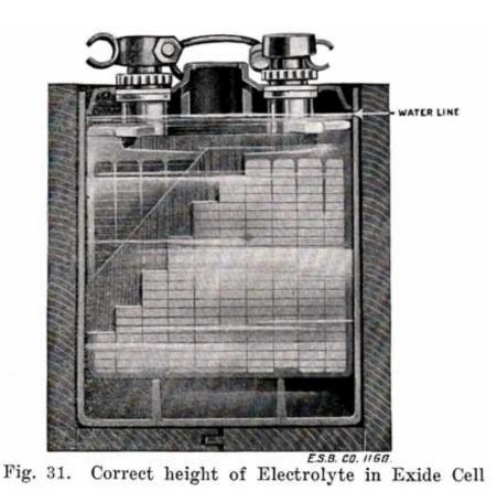
A convenient method of adding the water to the battery is to draw some up in a hydrometer syringe and add the necessary amount to the cell by inserting the rubber tube which is at the lower end into the vent hole and then squeezing the bulb until the required amount has been put into the cell.
