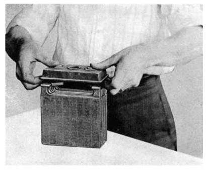
Fig. 250. Removing Prest-O-Lite Cover
