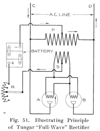
The rectifier shown in Figure 50 is a "half-wave" rectifier. That is, only one-half of each alternating current wave passes through it to the battery. If two bulbs are used, as shown ill Figure 51, each half of the alternating current wave is
