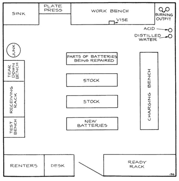
Fig. 136. Layout for a Small Shop
