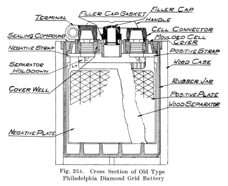
Figs. 254 and 255 show the construction of the old type Philadelphia Diamond Grid. Battery. Figs. 254 and 256 show the diamond shaped grid from which the battery derives its name. It is claimed that this construction gives a very strong grid, holding the active materials firmly in place, and giving a large amount of contact surface between the grid and the active material.
