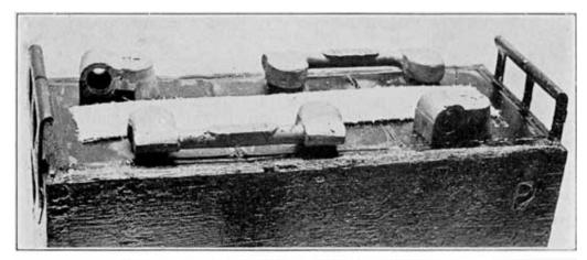
Fig. 147. Connectors "Burned" to Posts
