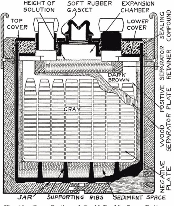
Fig. 10. Cross-Section of Gould Double Cover Battery
