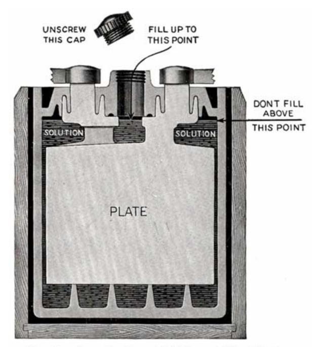
Fig. 13. Cross Section of Old Type Willard Battery
