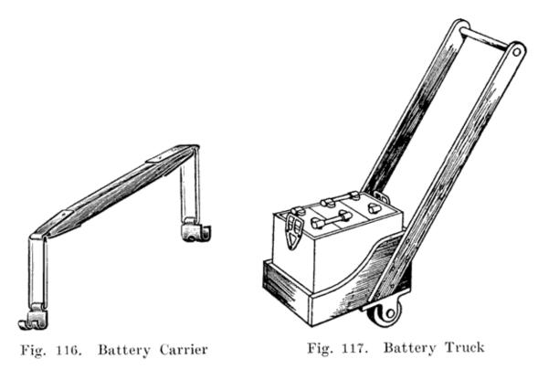
**Battery Carrier**. Figure 116 shows a very convenient battery carrier, having a wooden handle with two swinging steel hooks for attaching to the battery to be carried. With this type of carrier no strain is put on the handle, as is the case if a strap is -used.
