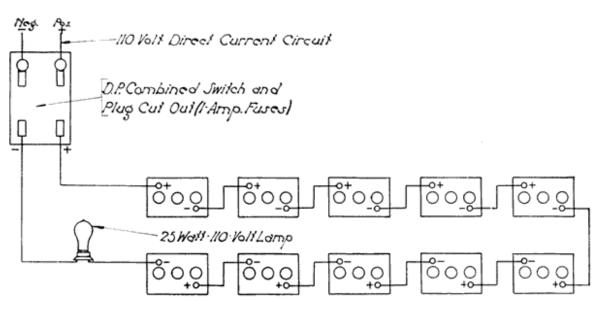
Fig. 151. Batteries Connected Up For "Trickle" Charge
