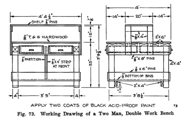
Figure 71 shows a single work bench which may be placed against a wall. Figures 72 and 73 show double work benches. Note that each bench has the elevated shelf, which should not, under any consideration be omitted, as it is absolutely necessary for good work. The tool drawers are also very convenient.
