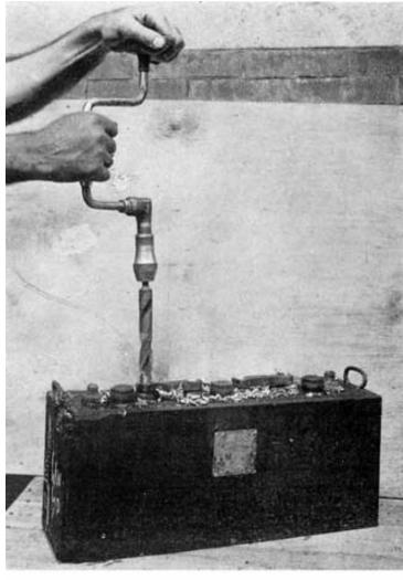
Fig. 191. Drilling Post and Cell Connector
