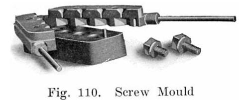
Figure 110 shows a Screw Mould which casts standard square lead leads on four screws in one operation, two 5/8 inch and two 3/8 inch. This mould has a screw adjustment in the base which makes each cavity adaptable to any length screw.
