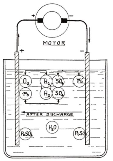
Chemical Action in a Storage Cell During Fig. 20 Discharge
