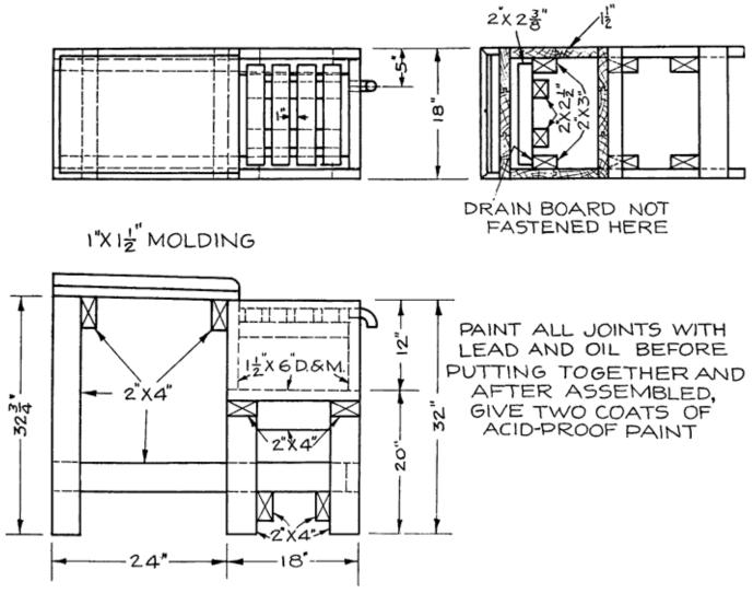
Fig. 76. Working Drawing of Wash Tank
