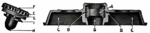
Sectional View of Cover, Plug Removed. Air Passages (BB) Closed and Air Lock (A) in Position to Prevent Overfilling Old Exide Cover
