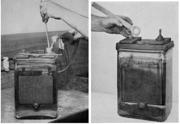
Fig. 319. Burning on Negative Strap. Delco-Light Cell
