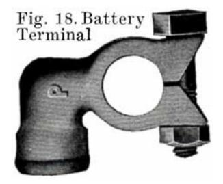
Many types of terminals are in two parts, one being permanently attached to the car circuit and the other mounted permanently on the battery by welding it to the terminal post, the two parts being detachably joined by means of a bolted connection.
