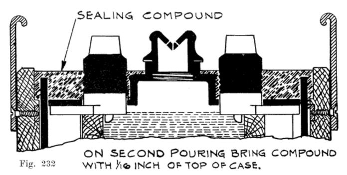
Fill the pouring ladle with compound, which is thinner than that used in the first pouring, and pour within 1/16 inch of the top of the case, being careful to get in just enough, so that-after it has cooled, the covers will press down exactly even with the top of the case, Fig. 232. It will require some experience to do this, but you will soon learn just how much to use.
