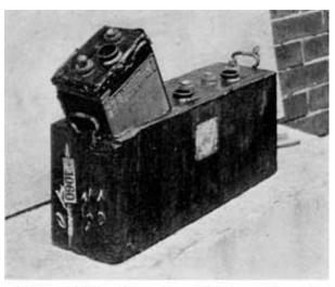
Fig. 197. Resting Element on Jar to Drain
