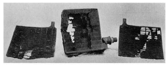
Fig. 210. Disintegrated Positives
