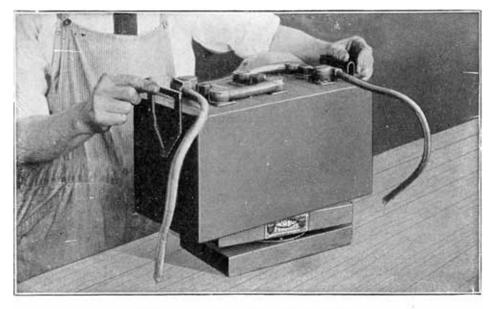
Fig. 111. Battery Turntable
