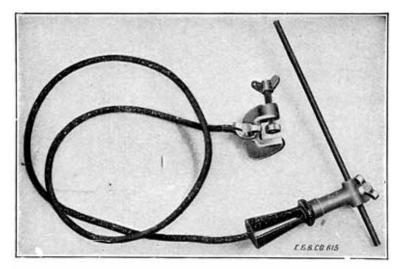
Fig. 80. Carbon Lead Burning Outfit
