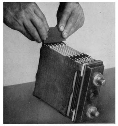
Fig. 269. Pressing Down Vesta Hard Rubber Isolator
