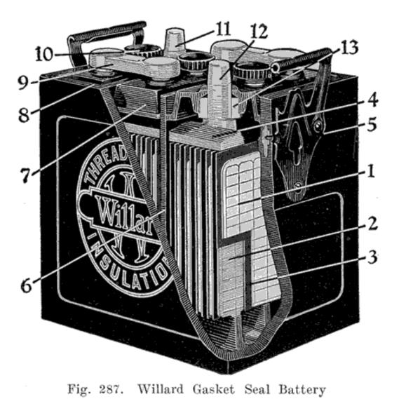
1. Drill off the connectors and terminals, leaving the post stubs, as high as possible, since the only way of removing the plates is by grasping the post stubs with pliers.
