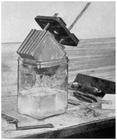
Fig. 307. Draining Element. Delco-Light Cell
