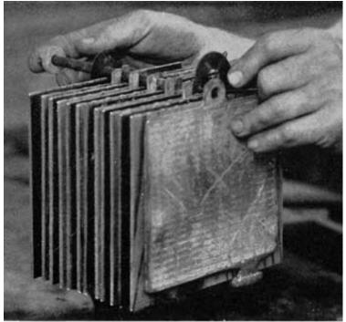
Fig. 208 Removing Cover of Deleo-Light Cell Fig. 200 Percent Look Din. Deleo Light Cell http://www.powerstream.com/1922/battery\_1922\_WITTE/batteryfiles/chapter17.htm (32 of 58) [5/11/2009 3:31:41 PM]
