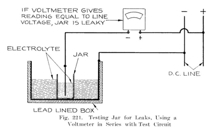
This test may be made by using a voltmeter instead of lamps, as shown in Fig. 221. If a voltmeter is used, be especially careful to have the part projecting above the liquid perfectly dry. A leaky cell will be indicated by a reading on the meter equal to the line voltage.
