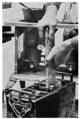
Fig. 234. Pressing Covers Down Around Posts to Make Them Flush With Top of Case
