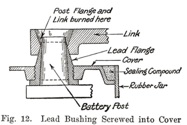
In older type U. S. L. batteries a bushing was screwed up through the cover, and then burned to the post and cell connector.
