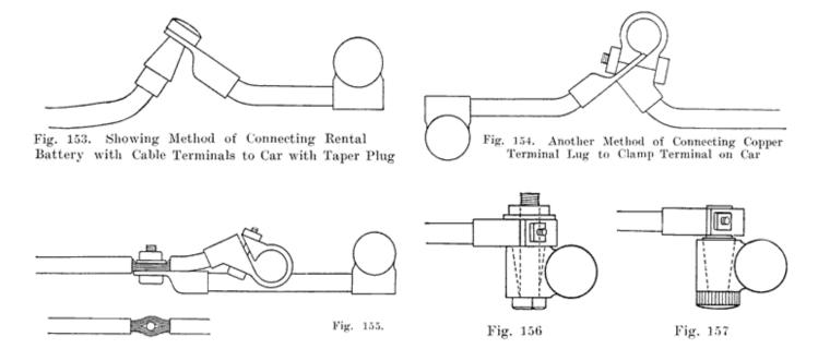
Fig. 155. Showing method of connecting rental batteries with cable terminals, to cars with clamp type terminals. In Fig. 155 the cable insulation is stripped for a space of an inch and the strands are equally divided with an awl. A bolt is passed through the opening and a washer and nut complete the connection.
