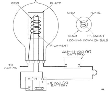
Fig. 159. Illustrating Principle of the Audion Radio Bulb
