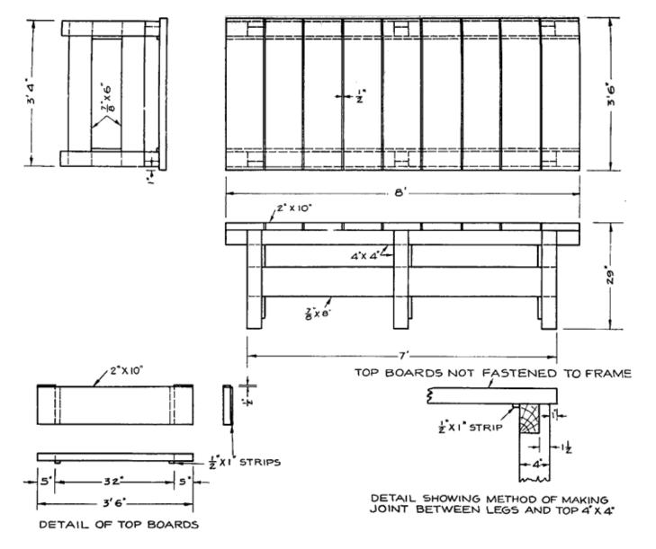
NOTE:-APPLY TWO COATS OF BLACK ACID-PROOF PAINT 67 Fig. 67. Working Drawing of Eight Foot Charging Bench
