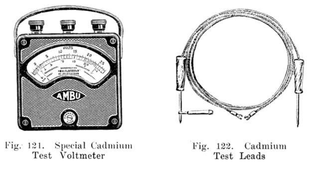
Cadmium tests may be made with any accurate voltmeter which gives readings up to 2.5 volts in divisions of .05 volt.
