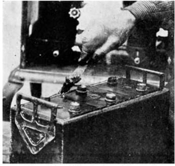
Fig. 237. Final Operation of Cleaning Off Excess Compound
