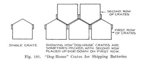
Some sort of a roof on a battery crate is required by law, the idea being to make it difficult to turn the crate up-sidedown. Perhaps the best crate would be one with a flat top marked "This Side Up," but such a crate would not comply with the law.
