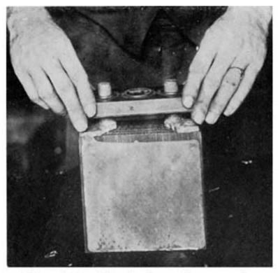
Fig. 258. Replacing Cover of Philadelphia Diamond Grid Battery
