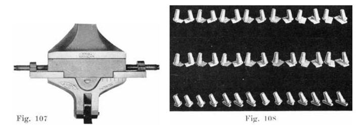
Figure 106 shows a production type strap mould which is designed to be used by large battery shops. Forty-two styles of straps are, cast by this mould. This mould has an indexing device as shown in Figure 107, which is adjusted by means of a screw for moulding the straps for any number of plates from seven to nineteen. Figure 109 shows some of tile castings which are made with this mould.
