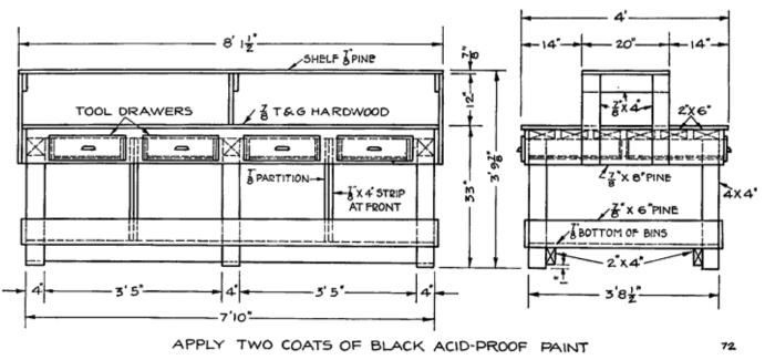
Fig. 72. Working Drawing of a Double, Four Man Work Bench, with Two Tool Drawers for Each Man
