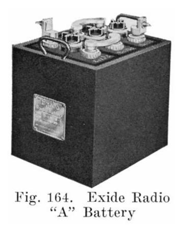
The Exide Radio "A" battery, Fig. 164, is made in four sizes, the capacities ranging from 20 to 120 ampere-hours. The design and construction of these batteries are similar to the Exide starting batteries. The over-all height of these batteries is approximately 95/8 inches, the width 7-5/16 inches, while the length varies with the number of the plates.
