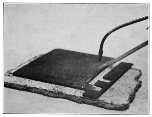
Fig. 150. Extending Lug on Plate
