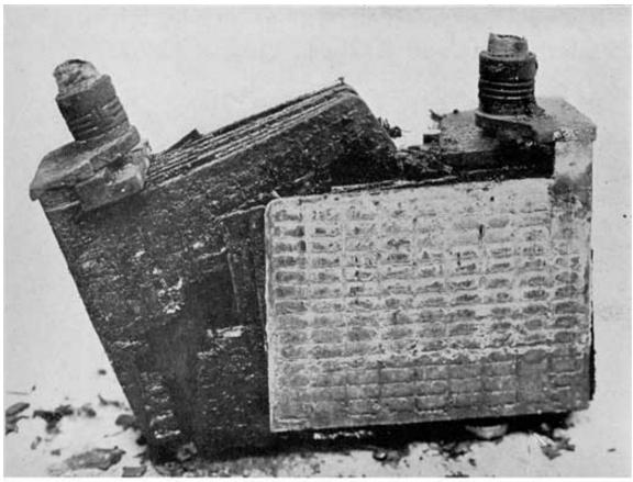
Fig. 209. Corroded, Bulged, and Sulphated Negatives. Disintegrated, Rotten Positives
