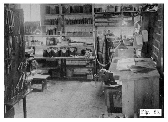
Fig. 83. Corner of Workshop, Showing Lead Burning Outfit, Workbench and Vises.
