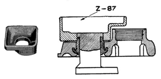
Fig. 283. Willard Burning Form Z-87, and How it Is Used
