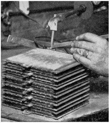
Fig. 322. Burning on Outside Negative Plate. Delco-Light Cell
