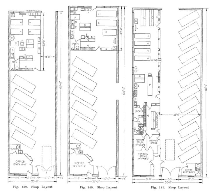
Fig. 139, 140 and 141: A- Receiving Rack. B-Power Drill. C-Wash Tank. D-Tear Down Bench. E-Hot Water Pan. F-Waiting Rack (6 Shelves). G-Repair Bench. H-Charging Table (3 Circuits). I-Electrolyte (10 Gal. Crocks). J-Separator Rack. K-Generator. L-Switchboard. M-Stock Bins. N-New Batteries. O-Live storage. P-Sealing Compound. R-Ready Rack (5-Shelves). S-Dry Storage. T-Torn Down Parts. (O and T in 141, not in 139 and 140.)
