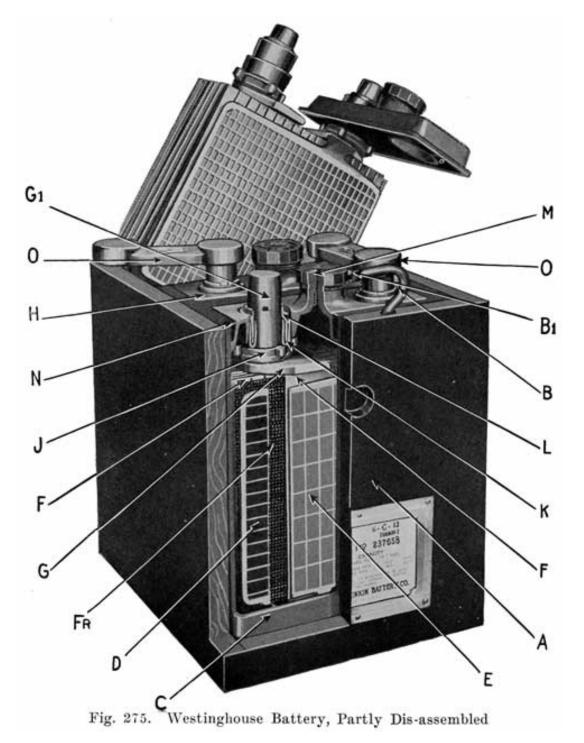
The lead sleeve is held in place by broaching or indenting the collar on taper lead sleeve into the posts.
