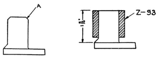
Fig. 281. Willard Post-Builder Z-93, and Built-Up Post
