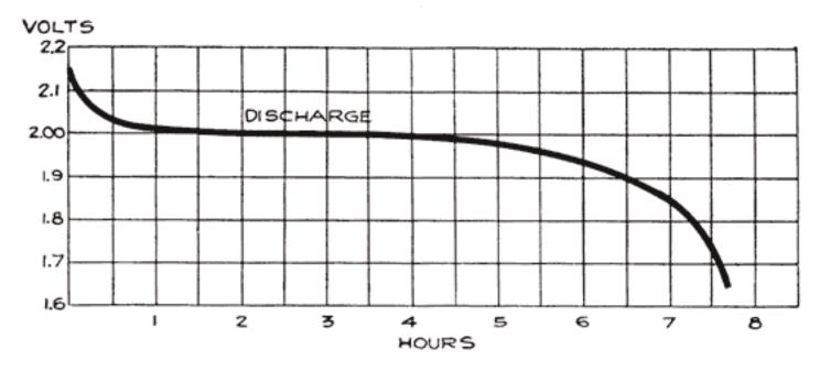
Fig. 22. Voltage Changes During Discharge
