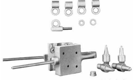
Fig. 109. Terminal Mould and Castings Made in It
