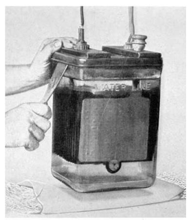
Fig. 306. Removing Delco-Light Cell Cover
