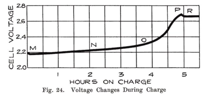
As shown in Fig. 24, the voltage remains almost constant between the points M and N. At N the voltage begins to rise because the charging chemical reactions are taking place farther and farther in the inside parts of the plate, and the concentrated acid formed by the chemical actions in the plates is diffusing into the main electrolyte. This increases the battery voltage and requires a higher charging voltage.
