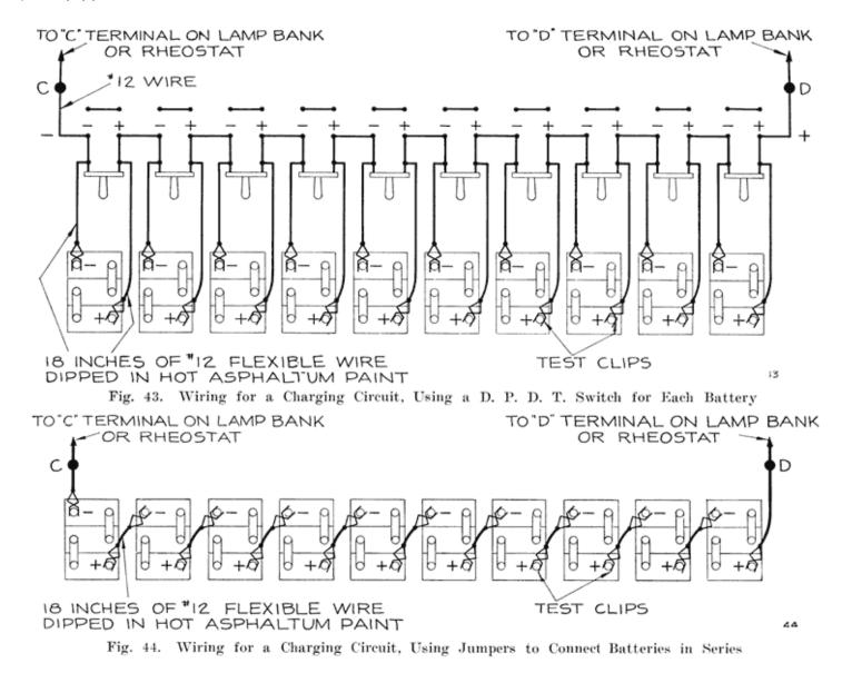
Figure 44 shows a ten-battery charging circuit. on which the batteries are connected in series by means of jumpers fitted with lead coated test clips, as shown. This layout is not as convenient as that shown in Figure 43, but is less expensive.
