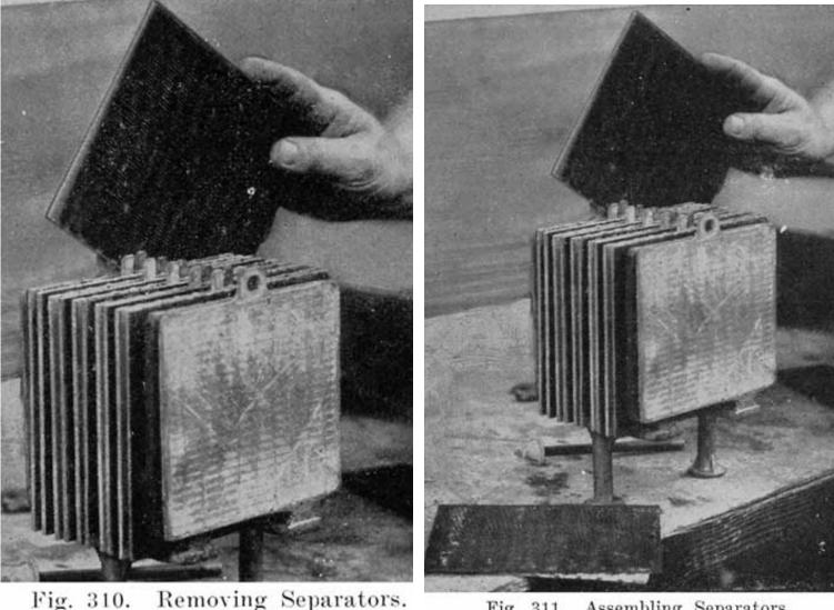
Fig. 311. Assembling Separators. Delco-Light Cell
