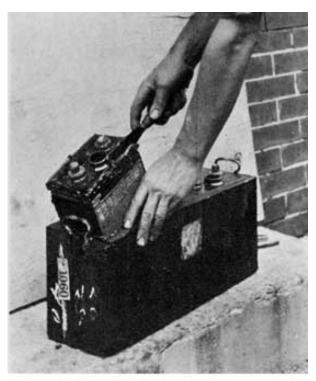
Fig. 198. Removing Compound from Cover
