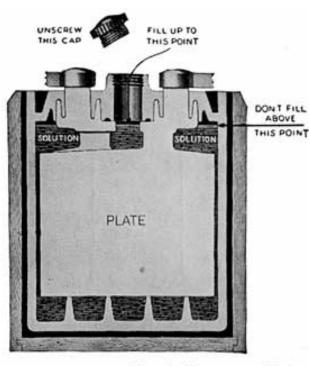
Fig. 277. Willard Battery Using Sealing Compound Around Posts
