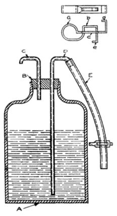
Fig. 133. Siphon for Drawing Acid from Carboy
