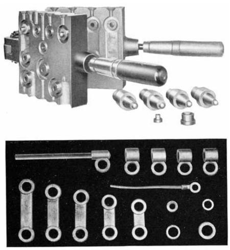
Figs. 103 and 104. Link Combination Mould, and Castings Made in It
