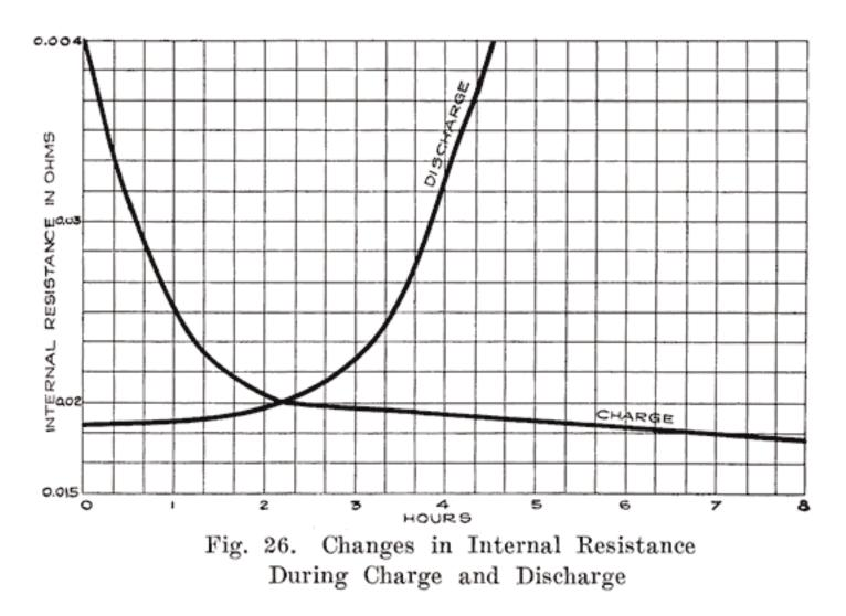
The resistance as measured between the terminals of a cell is made up of several factors as
