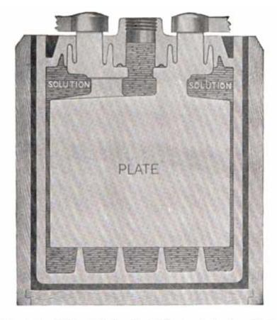
Fig. 32. Cell with level of Electrolyte too high
