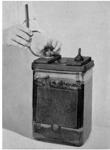
Fig. 321. Fastening Auxiliary Strap. Delco-Light Cell
