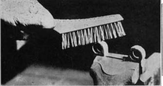
Fig. 143. Brushing Connector Before Burning In
