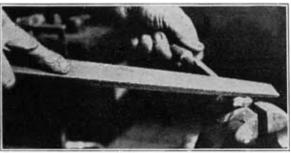
Fig. 144. Rasping Connector Before Burning In
