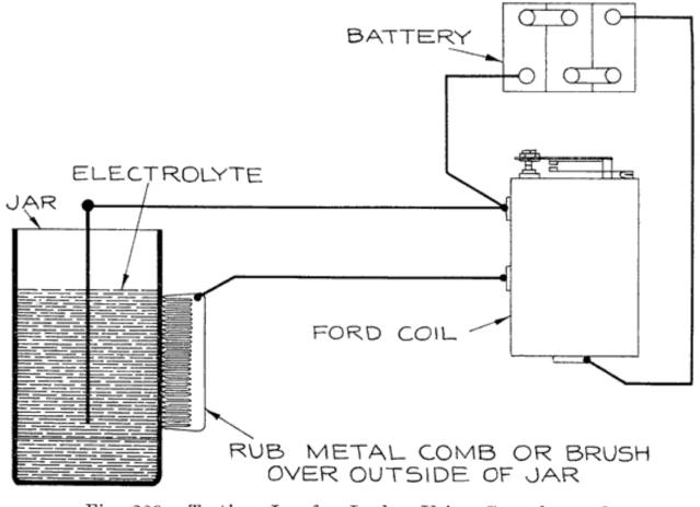
Fig. 223. Testing Jar for Leaks, Using Secondary of Ford Ignition Coil, or Any Other Vibrator Ignition Coil
