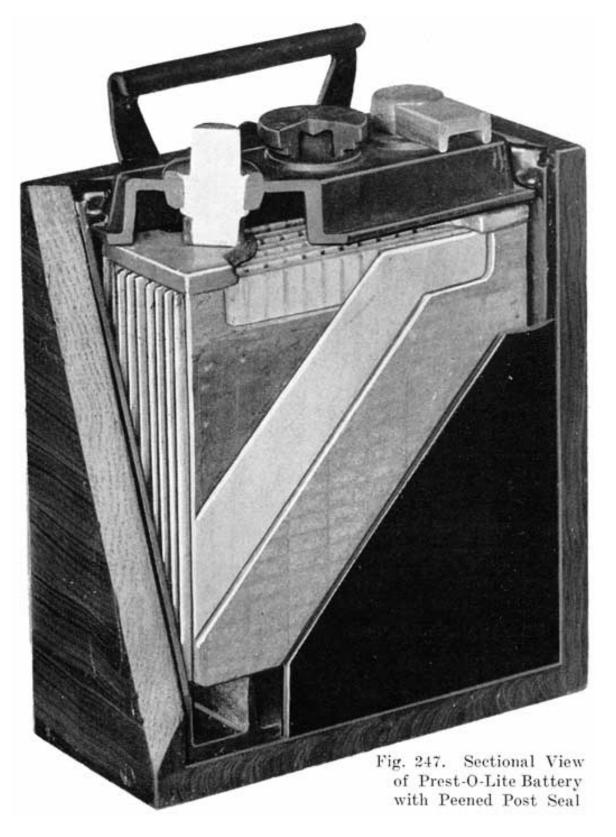
However, where the cover is broken or must be replaced for other reasons, when plates have to be renewed, or the posts have been broken off below the cover, the element and cover must be separated.
