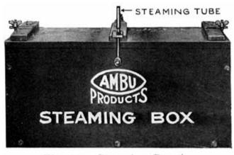
Fig. 93. Steaming Box in Which Entire Battery is Set
