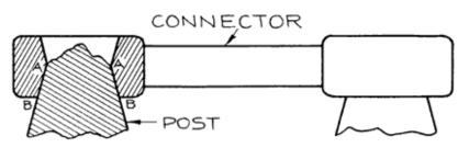
Fig. 146. Connector in Position on Post for Welding to Post. Surfaces A-B Are Not Welded Together
