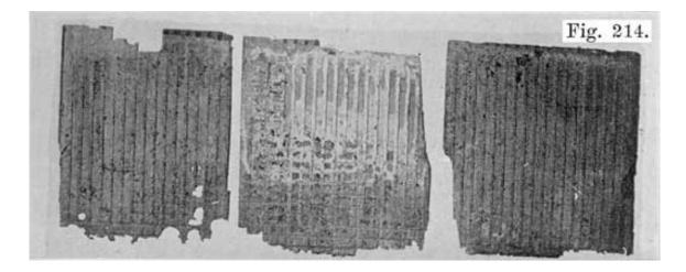
Fig. 214. Separators Worn Thin and Cut Through on Edges by Buckled Plates. Holes Worn Trhough by Bulged Active Material, Center One Shows Cell Was Dry Two Thirds of the Way Down.
