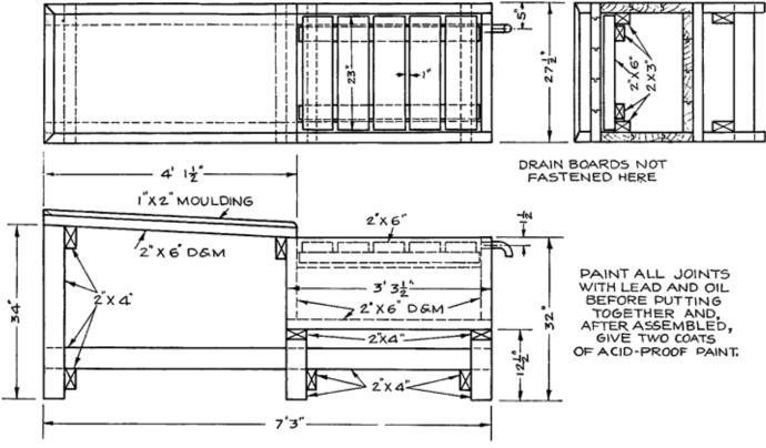
Fig. 77. Working Drawing of a Wash Tank
