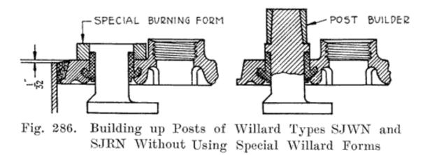
6. Set post builders on the part of the posts which has been built up and build up the posts as usual, Fig. 286. Then burn on the connectors and terminals.
