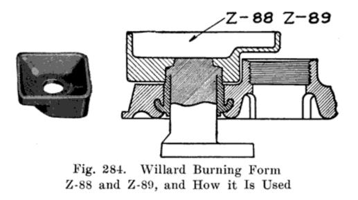
10. Now seal the covers with sealing compound as usual, and burn on the connectors.
