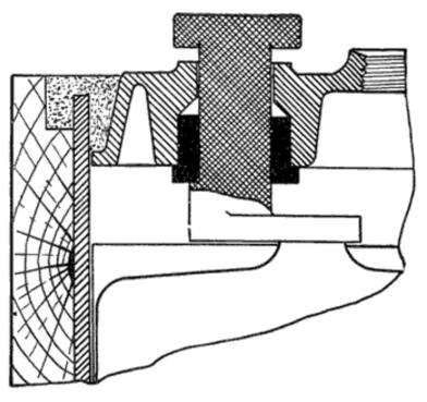
Fig. 288. Details of Willard Gasket Seal
