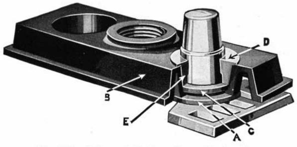
Fig. 291. Universal Battery Cover Construction
