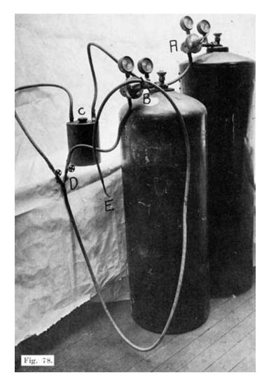
Fig. 78. Hydrogen-Oxygen Lead Burning Outfit. A and B are Regulating Valves. C is the Safety Flash Back Tank. D is the Mixing Valve. E is the Burning Tip.
