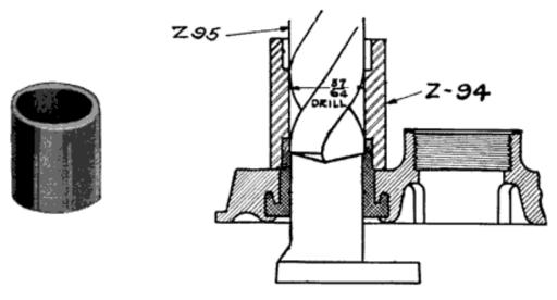
Fig. 280. Willard Jig Z-94, and How it Is Used
