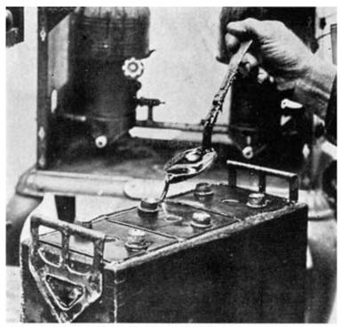
Fig. 236. Filling Cracks Around Covers With Sealing Compound
