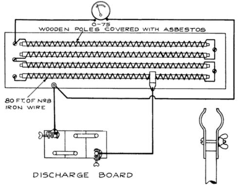
Fig. 180. Simple High Rate Discharge Rheostat
