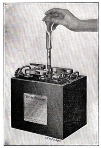
Fig. 35. Taking a Specific Gravity Reading
