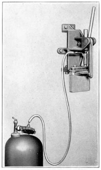
Fig. 248. Special Prest-O-Lite Peening Press
