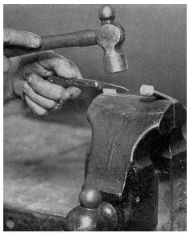
Fig. 318. Splitting End of Strap. Delco-Light Cell
