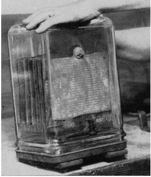
Fig. 315. Sealing Jar of Delco-Light Cell
