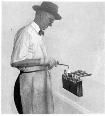
Fig. 251. Building up Posts on Prest-O-Lite Element
