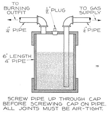
Fig. 79. Flash-Back Tank for Lead Burning Outfit
