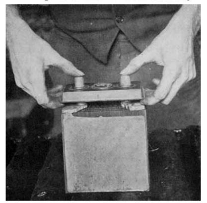
Fig. 259. Removing Cover from Philadelphia Diamond Grid Battery
