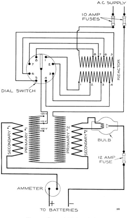
Fig. 58. Internal Wiring of the Four Battery Tungar Rectifier
