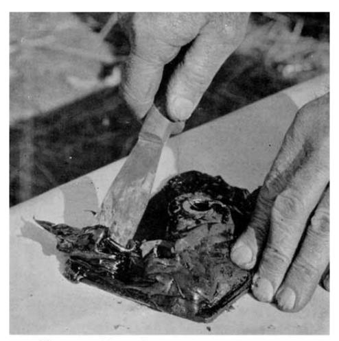
Fig. 199. Removing Sealing Compound from Double Cover
