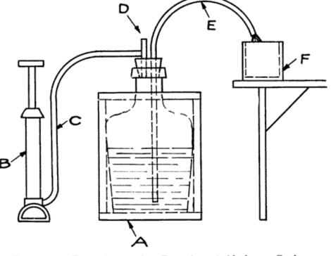
Fig. 134. Foot Pump for Drawing Acid from Carboy
