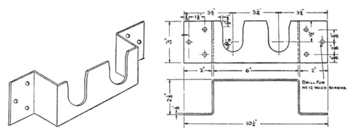
Fig. 289. Cover Removal Frame for Willard Gasket Seal Battery
