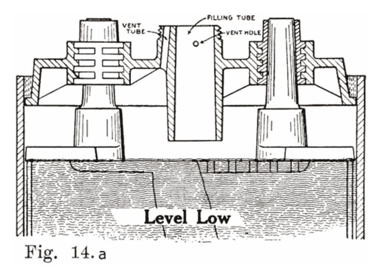
Several devices have been developed to make it impossible to overfill batteries. This has been done by the U. S. L. and Exide companies on older types of batteries, their constructions being described as follows:
