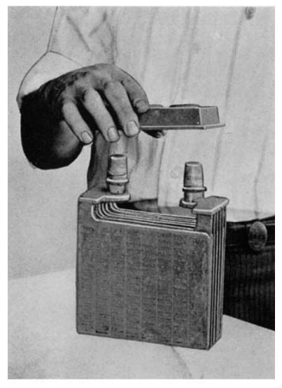
Fig. 252. Replacing Prest-O-Lite Cover on Built Up Posts
