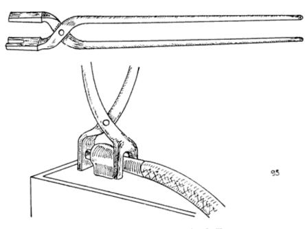
Fig. 95. Battery Terminal Tongs
