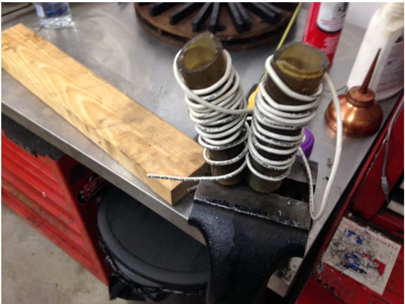
A magnet charger is made using one of our magnets clamped in the vice. I put a piece of
