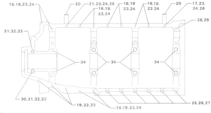
Figure 3. Propeller Governor Drive and Crankcase Attaching Parts
