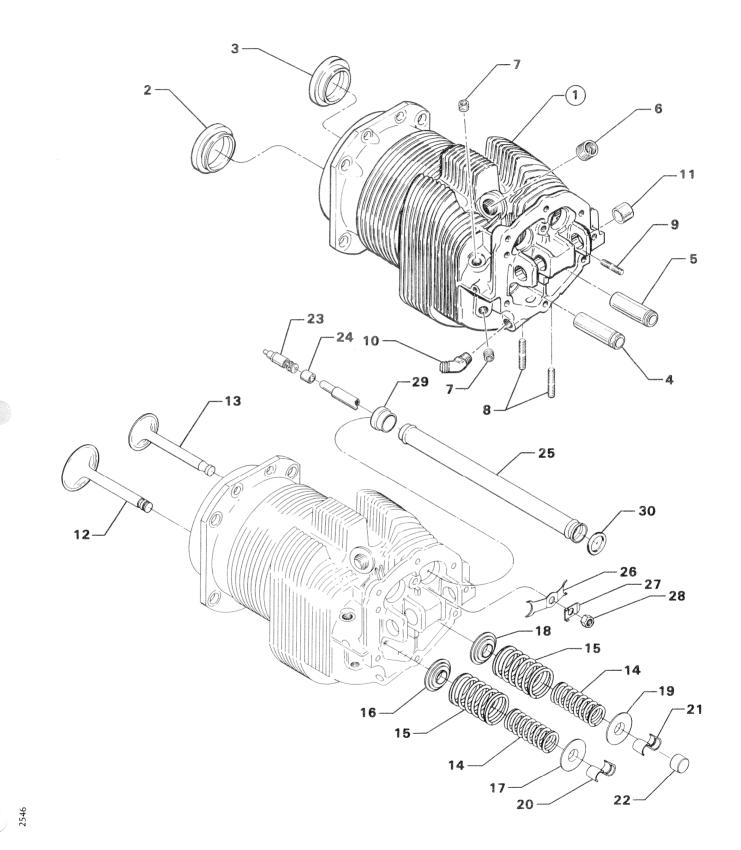
Figure 6. Cylinder, Valve Assembly and Attaching Parts
