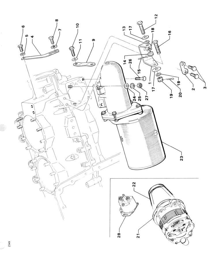
Figure 9. Starter, Alternator and Attaching Parts
