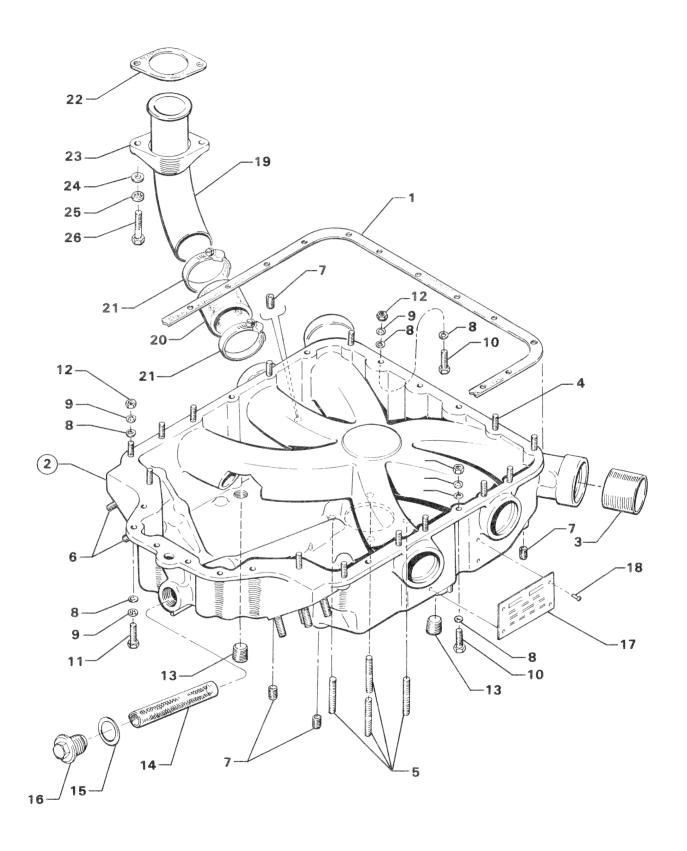
Figure 10. Oil Sump Assembly, Intake Pipes and Attaching Parts
