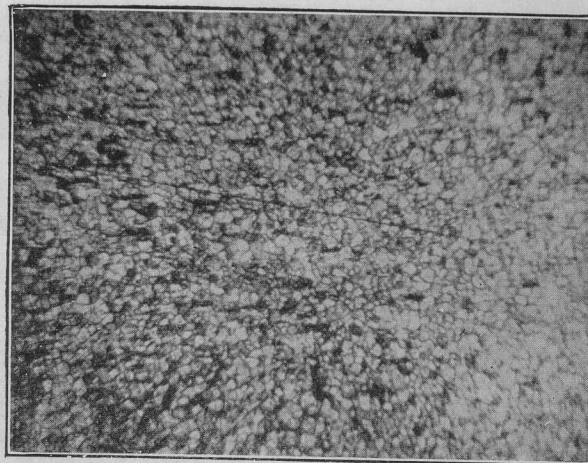
Fig. 4.—Micro-Section Photo of a 50 Per Cent. Tungsten-Molybdenum Alloy Briquet.
