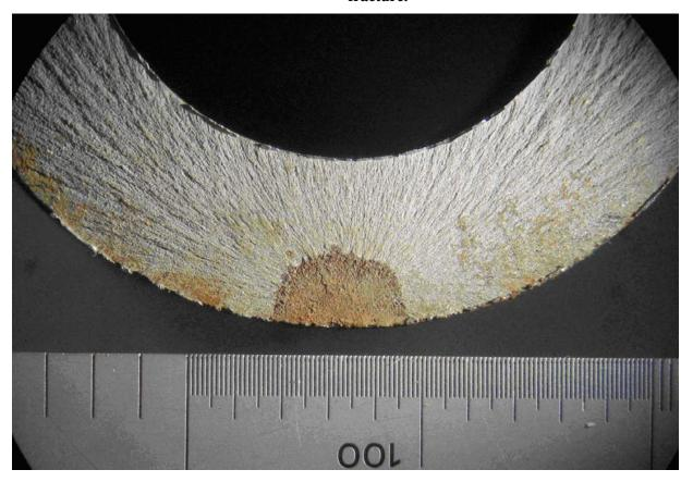
Photo 3: A tilted magnified view of the fracture surface showing pitting corrosion coincident with the area at the origin of the fracture.
