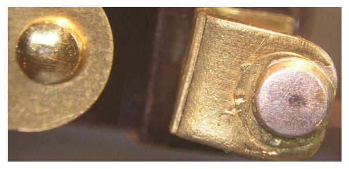
The photo above is typical of the N.C. contacts of both the failed and normally operating switches. The contact on the right shows some darkening in the interior of the arcing pit but neither contact shows metal transfer.
