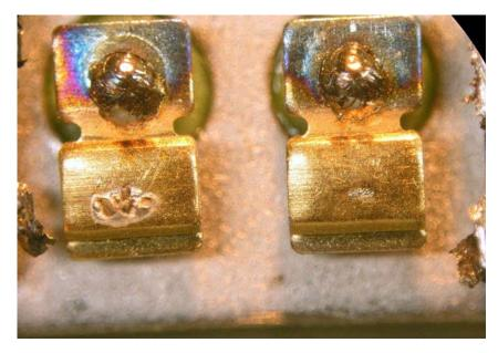
This is a view of the stationary contacts on the same relay. Metal transfer on the 27K cycle contact is profound.
