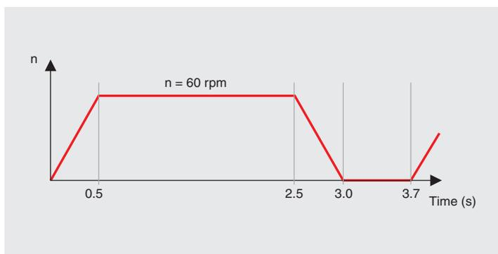
The inertia of load  $J_L$  to be accelerated is 130 000 gcm<sup>2</sup>. The constant friction torque is 300 mNm. The motor is to be driven with the linear 4-Q servo amplifier from maxon (LSC). The power supply delivers max. 5 A and 24 V.
