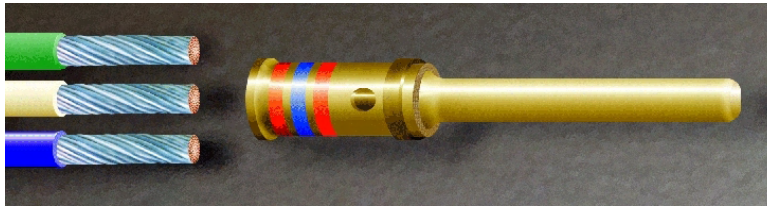
Figure 19-20. Stripped Wires Prior to Insertion
