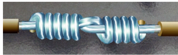
Figure 19-16. Completed Wrap for Western Union/Lineman Splice
