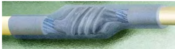
Figure 19-11. Sleeved Lash Splice
