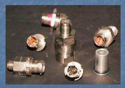
On Premier EEDs were used to initiate ignition of high power gas generator that deployed the parachute from the canister.
