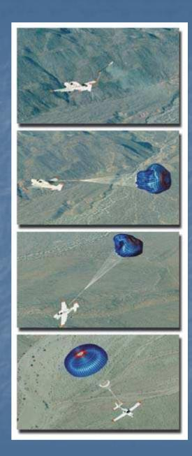
Simplest designs used combinations of springs to eject a drogue which in turn dragged a canopy from the canister on the tail of the aircraft.
