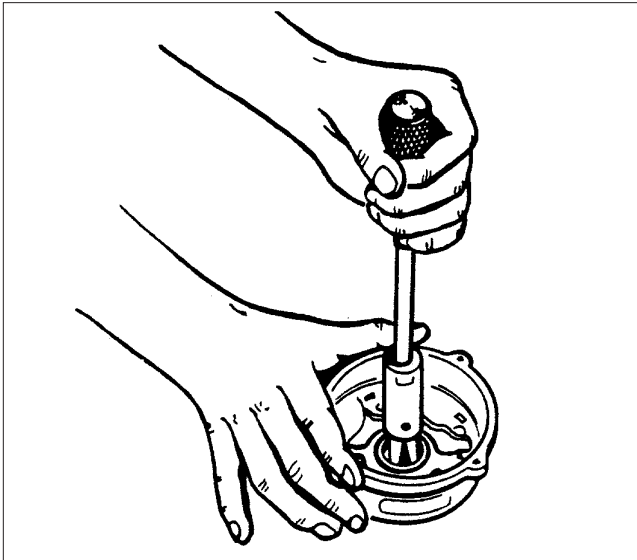
Removal of Slip Ring End Bearing Figure 5
