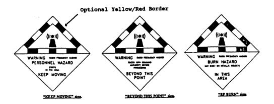
Figure 7-1. RF Hazard Warning Sign Format
