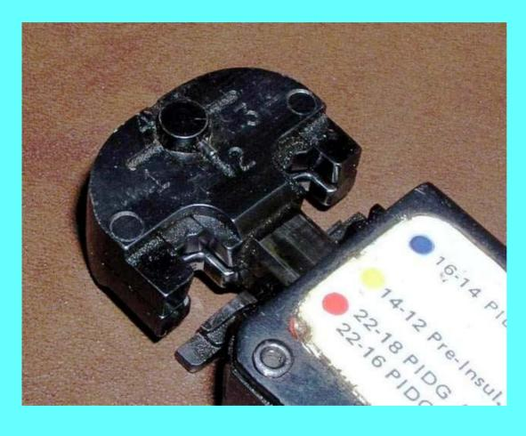
• The T-head tool offers ratchet handles and insulation grip, die-height adjustment.
