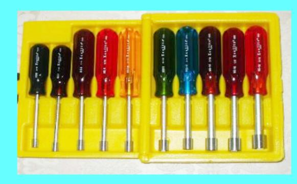
• Color coded hex nut drivers in sizes 1/4" to 9/16" are very handy compared to a loose socket stuck on the end of a handle.
