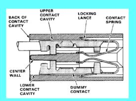
• Legacy avionics along with most strobe systems use the "open barrel" sheet metal pins that require some specialty tools for installation and maintenance.
