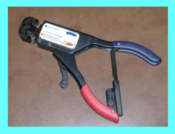
• This is the first tool in every professional aircraft electrician's toolbox.... The AMP "T-Head PIDG" crimper.
