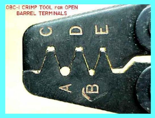
• Note that openings C, D and E have the sculptured die that fold wire grip tabs of the sheet metal pin over onto the wire.
