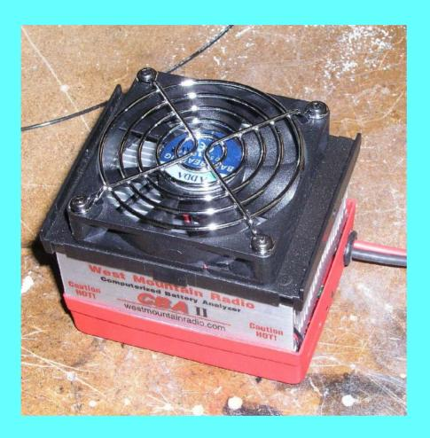
• The folks at West Mountain Radio offer this very capable computer driven battery capacity measurement system.
