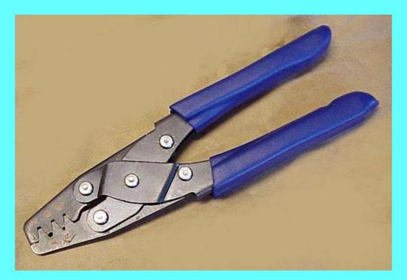
• This tool offers the range of b-crimp dies needed to install the open barrel, sheet metal pins . . .
