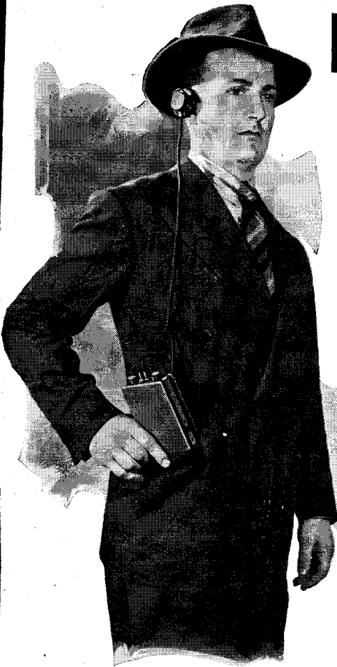
You can stow this midget receiver in a coat pocket. Note the parts arrangement at the right. Cigar-box wood forms the cabinet, and a loop antenna is wrapped around it, while flash-light cells to power the set are carried in the base
