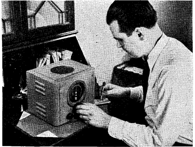
This two-tube superhet gives loudspeaker reception of local stations with a 20-foot antenna laid on the floor
