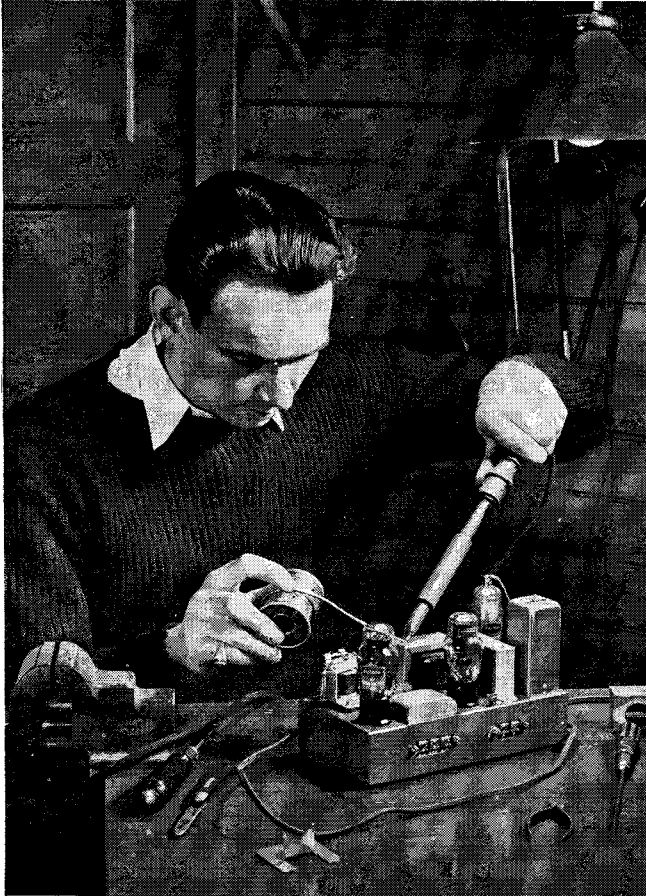
All connections must be soldered carefully, and a metal shield, as at the right, must be used to eliminate radio interference
