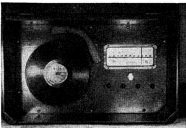
Top view showing phonograph turntable, radio dial, and controls
