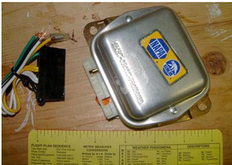
Standard regulator, available from many parts stores.
