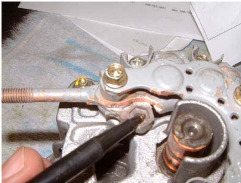
With the copper portion of the tab removed, the plastic nut retaining pocket is next. But first, make a mark down through this nut pocket, into the chassis, to accommodate the next photo.
