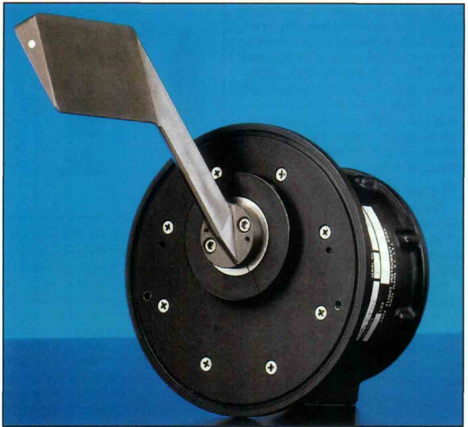
Photo A - Safe Flight Instrument's AOA vane used on large aircraft.
