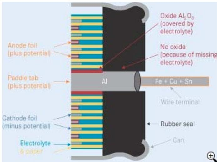
FIGURE 2: PARTIAL FORMING IN THE TERMINAL AREA
