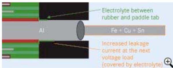
FIGURE 3: REFORMING IN THE TERMINAL AREA
