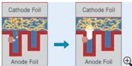
Every change in equilibrium that affects the gas and electrolyte quantity and its gaseous solubility can cause the leakage current to rise. This also explains the paradoxical observation that even when a capacitor cools, the leakage current can initially rise contrary to expectations.
