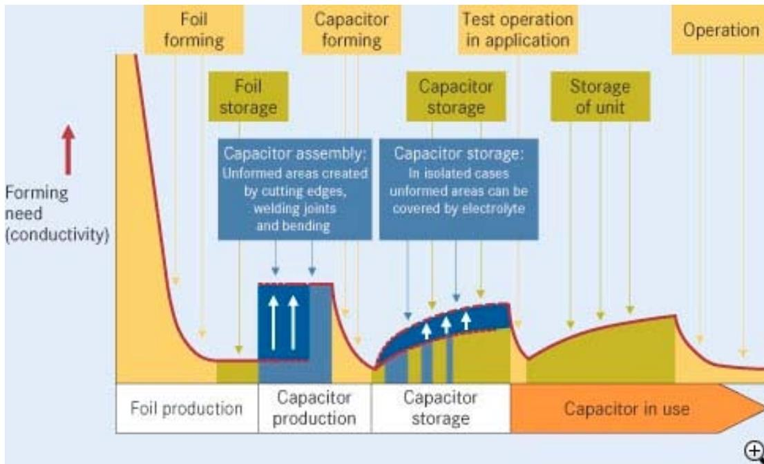
FIGURE 1: LEAKAGE CURRENT OF ALUMINUM ELECTROLYTIC CAPACITORS
