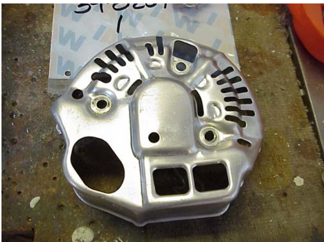
This last picture above shows the back cover removed with the brush assembly, internal regulator and rectifier exposed. This is removing the three nuts and one ground lug on the back cover. Note: the area of the back cover below that has two square holes internal regulator will need to be modified to allow the terminal posts to come out there.
