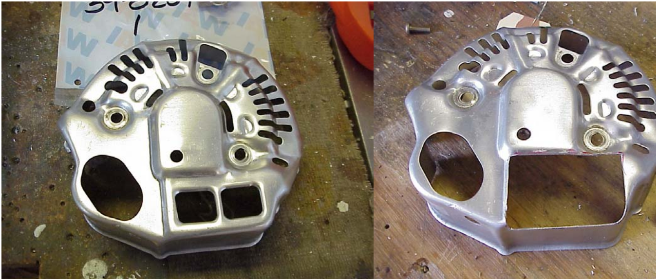
This shows the rear cover modified to fit the terminal block.
