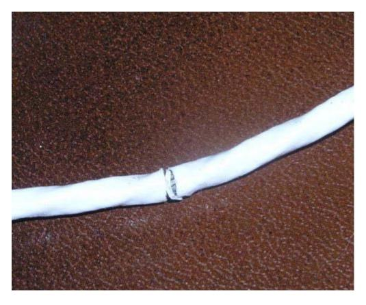
Tefzel jackets are also very thin. PVC insulation is thick enough that 'pushing' a strip-length off at the cut tends expand the inner diameter of the insulation lessening the grip on the wire. Tefzel is so thin that the same push fails the insulations column strength in compression and it simply bunches up . . . and rips the shield strands but still hasn't budged in the space beyond.
