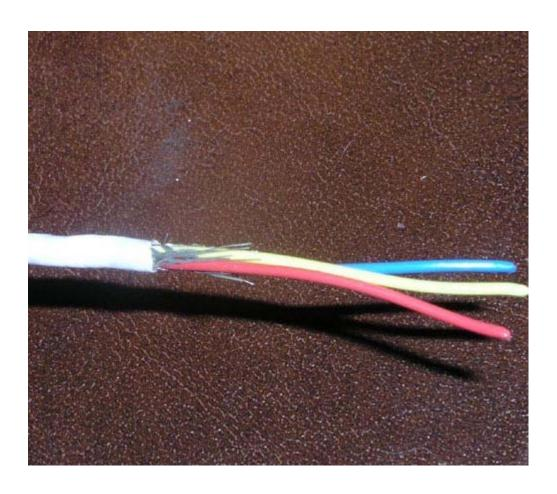
You wind the shield remnants tightly around the wires like this . . . keep the diameter small.
