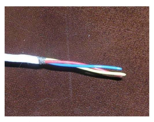
If the wire is 'old' . . . the shield strands may be less than bright. Optionally, you can prepare the strands to accept a solder sleeve by 'tinning' them but shake off all excess solder.
