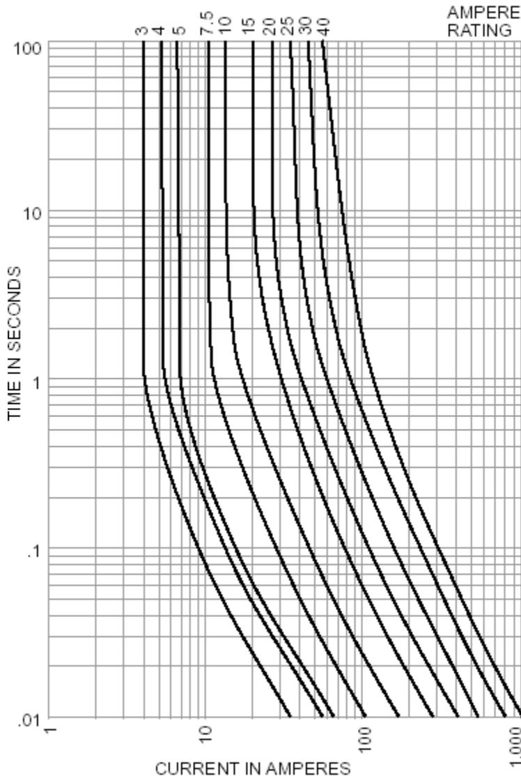
Note that the blowing time for a 3-amp ATC fuse goes asymptotic (parallel) to infinite blowing time at 4-amps. This tells me that the manufacturer of the device is guaranteeing me that his 3-amp fuse will be just fine running at 100% of it's rated value and that he has ALREADY de-rated it about 25% to insure predictable performance.
