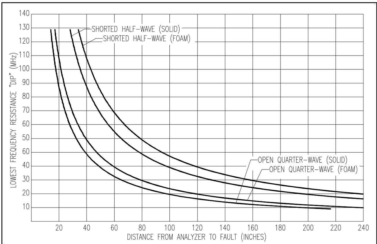
There are two curves each for the "shorted" and "open" condition. One curve represents the characteristics of coax cable with a solid plastic insulation between the center conductor and the shield. The other curve is for coax with foam insulation.
