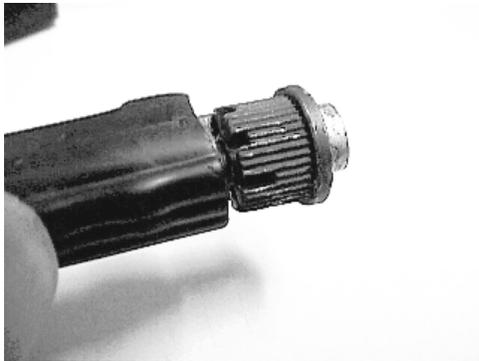
**Crimp Adjust:** This knob can be pulled out to disengage locking slots and rotated to size the finished crimp. Rotating clockwise increases size, counter-clockwise decreases size.
