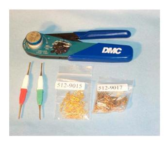
Daniels and others make some fine tools . . . most conform to industry and military specifications for the installation of machined pins for d-sub, AMP circular
