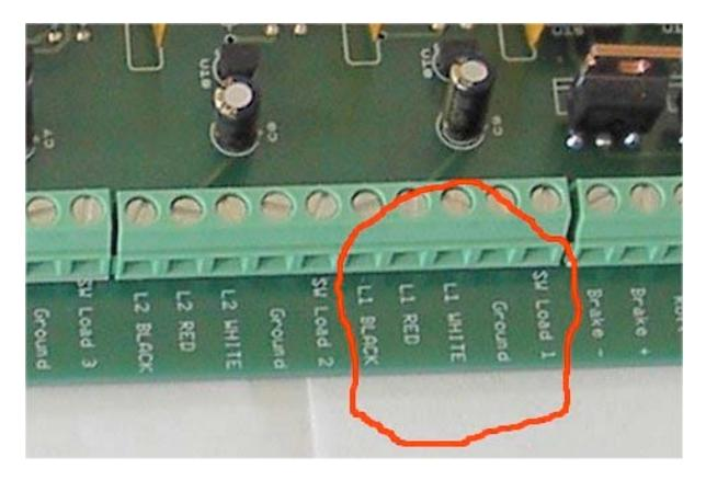
The circled are shows Switched Load 1, which is labeled SW Load 1 and Ground.
