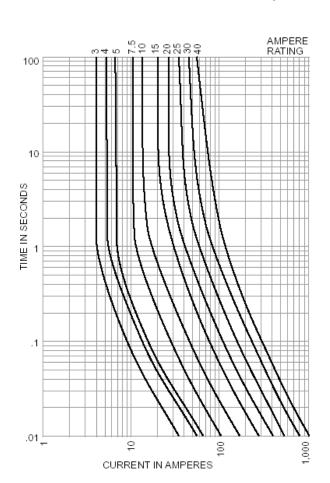
or breaker won't hold above 80% of what it says on the nameplate; so a 50 Amp breaker will pop at 40 amps after 20 or 30 minutes. Just long enough into the flight to be a bother!
